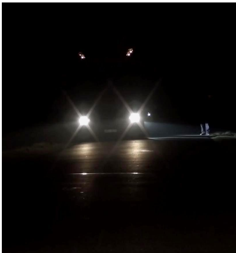
Fot. 2. Side illuminating lamp perfectly illuminates pedestrian's leg even in black trousers.
