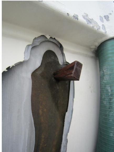
The dark grey area with the plug is the protective lining, the light grey colour is the aluminium alloy shell material and the peeling off white/grey is the paint.
