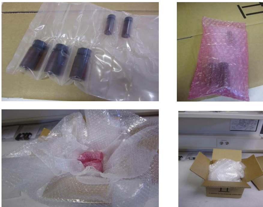
Figure 3 Placement of sample vessel in secondary package
