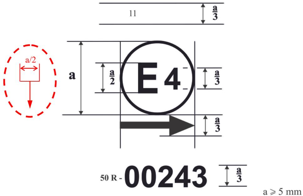
A device bearing the approval mark shown above is a direction indicator of the category 11 approved in the Netherlands (E4) under the number 00243. The first two digits of the approval number indicate that the approval was granted in accordance with the requirements of Regulation No. 50 in its original form.
