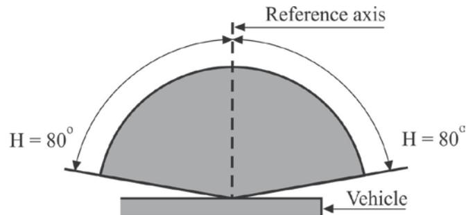
Front position lamps (for a pair of lamps)
