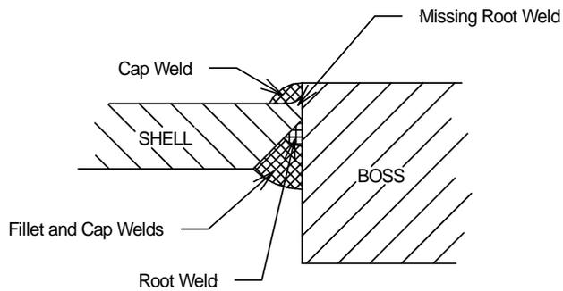
This missing weld gave an indication, during the MPI examination, that an internal crack was present along the length of the missing weld.
