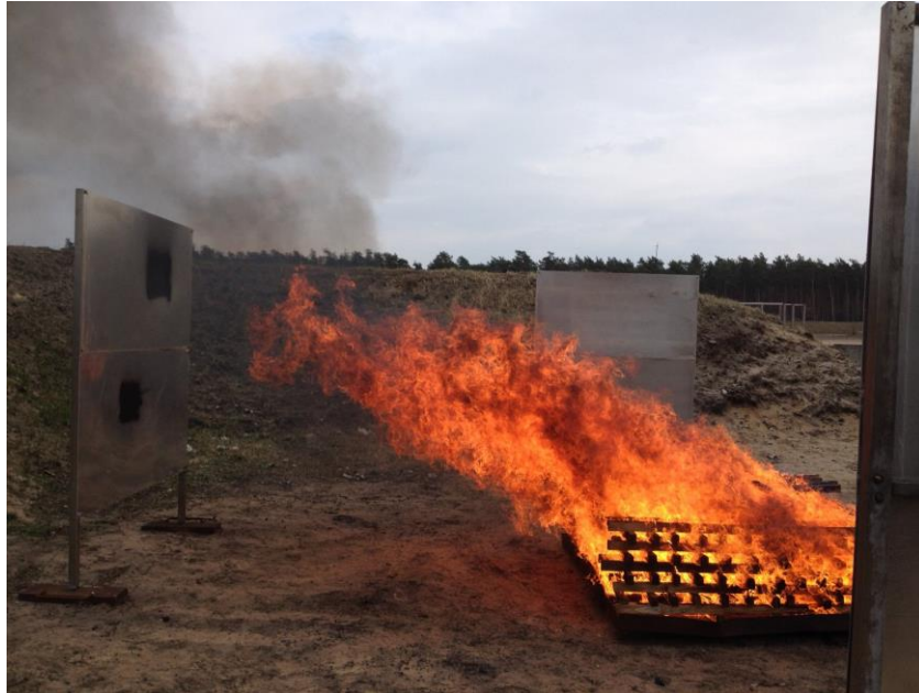
Fig. 6: Conditions at wind speed of 6.6 m/s
