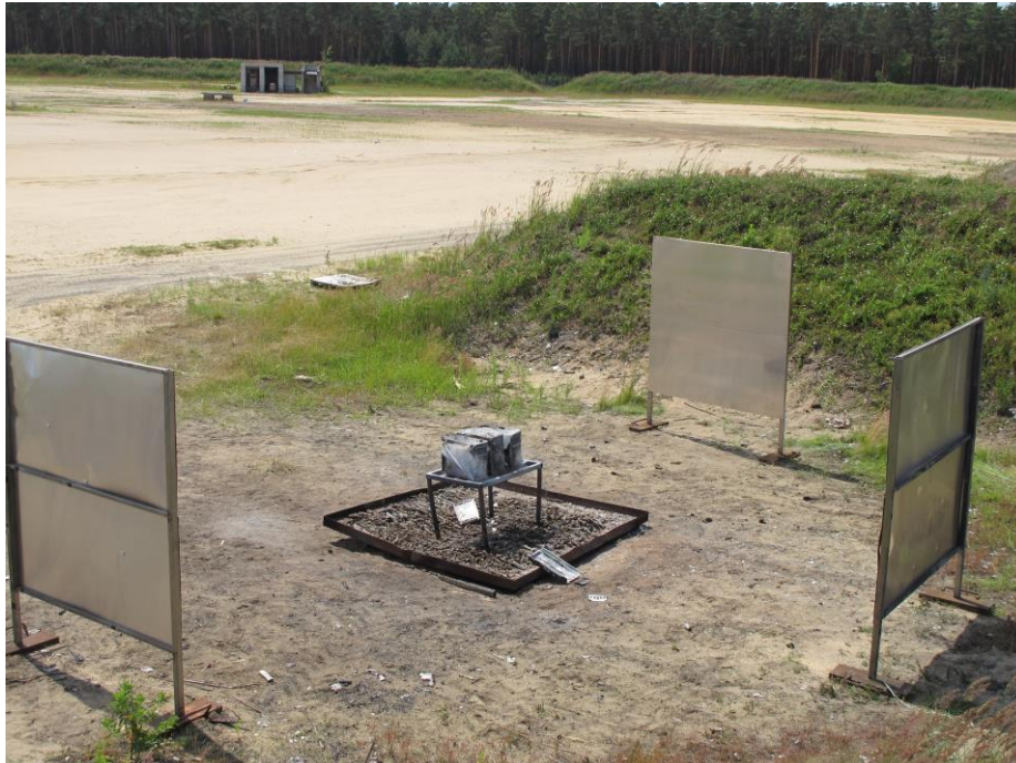
Fig. 1: Overview of the 6(c) test after the test performance
