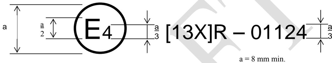
The above approval mark affixed to a vehicle shows that the vehicle type concerned has, with regard to its pole side impact performance, been approved in the Netherlands (E4) pursuant to Regulation No. [13X] under approval number 01124. The approval number indicates that the approval was granted in accordance with the requirements of Regulation No. [13X] as amended by the 01 series of amendments.
