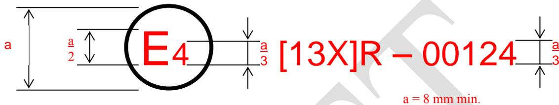
The above approval mark affixed to a vehicle shows that the vehicle type concerned has, with regard to its pole side impact performance, been approved in the Netherlands (E4) pursuant to Regulation No. [13X] under approval number 00124. The approval number indicates that the approval was granted in accordance with the requirements of Regulation No. [13X] in its original form.
