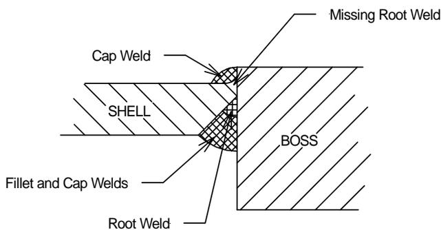
This missing weld gave an indication, during the magnetic particle inspection, that an internal crack was present along the length of the missing weld.
