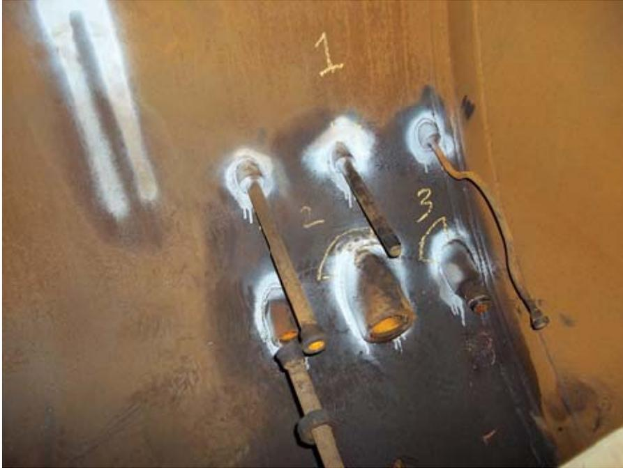
17. Following the initial indications of cracking light grinding of the surface was undertaken to ensure that it was not just weld overlap, however it was confirmed that all three were hairline cracks (the white background paint and black indicator has now made these very visible to the naked eye).
