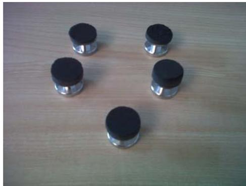
*Example of blocks with polyurethane material layer extracted (adhesion test)*
