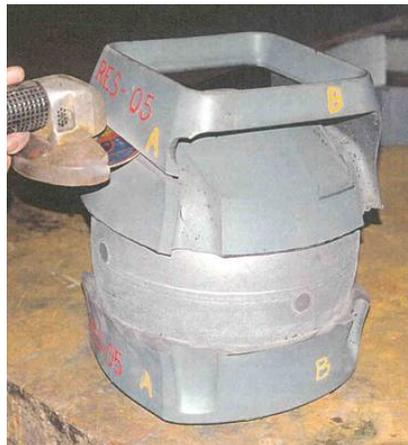
*Example of peeling test: the over-moulded material is peeled and the steel surface is inspected.
