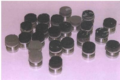
Example of blocks with polyurethane material layer extracted (adhesion test).
