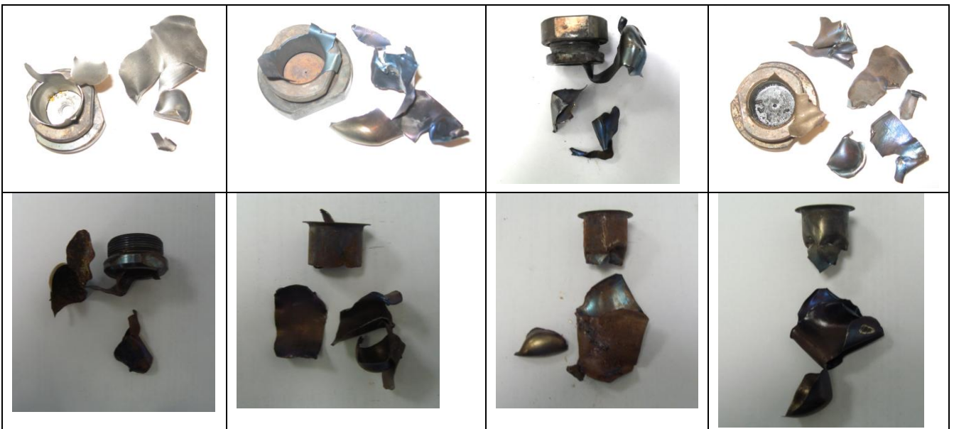
“F”: Tube fragmented into three or more mainly large pieces which in some cases may be connected with each other by a narrow strip;
