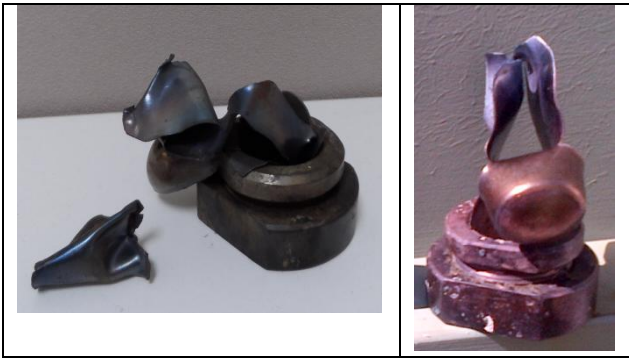
“F”: Tube fragmented into three or more mainly large pieces which in some cases may be connected with each other by a narrow strip;
