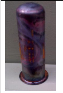
"A": Bottom of the tube bulged out
