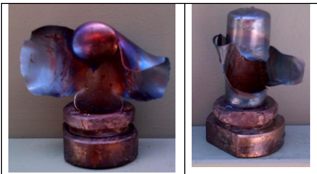
"D": Wall of tube split
