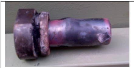
"B": Bottom and wall of the tube bulged out
