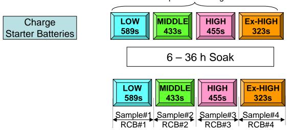
1 PM-Filter for all 4 phases, some labs to measure 2 Filters (L+M, HxH), SoC for each phase separately
