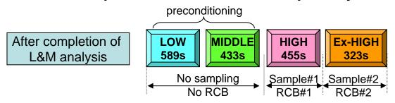
1 PM-Filter for all 4 phases, some labs to measure 2 Filters (L+M, HxH), SoC for each phase separately
