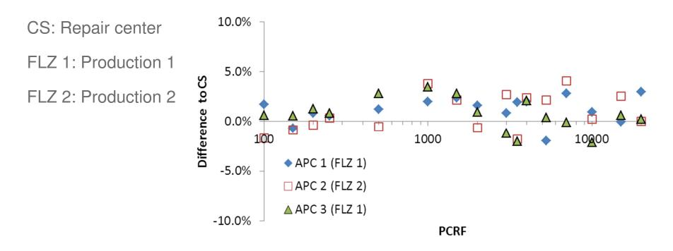
Three APCs were calibrated either at the CS (repair center) or the production lines 1 (FLZ 1) and 2 (FLZ 2). The mean differences were 1% and the 95% of the differences within 4%.
