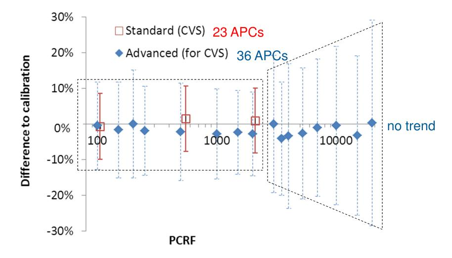
Recalibration of five VPRs (APCs from AVL) units after many months of use at the CVS Error bars show 2 standard deviations.
