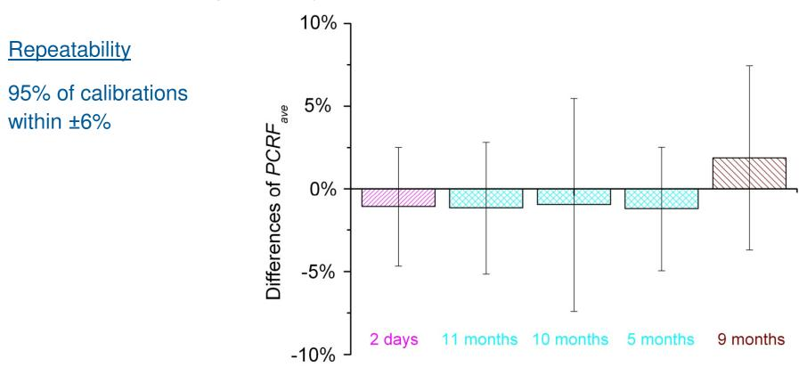
Recalibration of five VPRs (APCs from AVL) units after two days (no modification), after 5-11 months (guidance rods and springs were changed) and after 9 months (rotating disk also changed).
