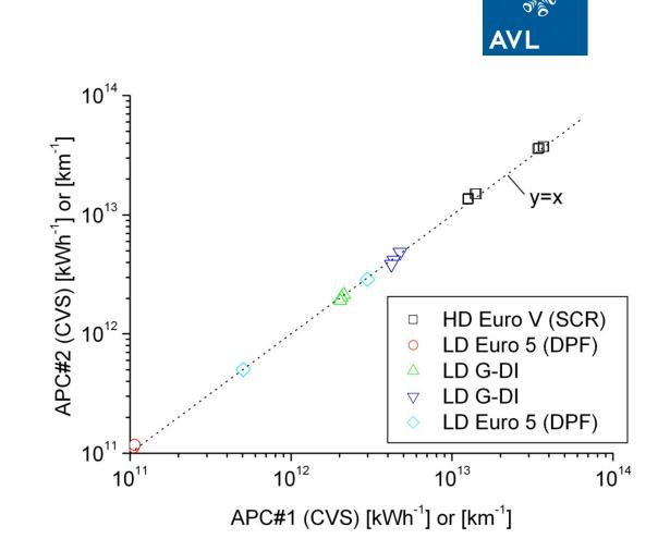
Comparison of two PN systems (APCs from AVL) both connected to the CVS for one heavy duty engine (different test cycles) and two different APCs for four different light duty vehicles (for the NEDC cycle).
