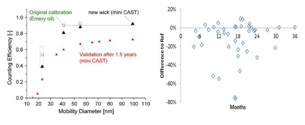
2 out of 5 drifted (40%) The reason is the wick (where the super-saturation is achieved) The critical point: **No light indicator identified this degrading**  New results: 15 out of 41 drifted (37%)
