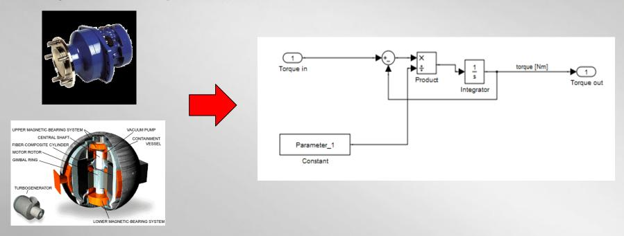
The result is a set of simulation models of non-electric powertrain components, which are suitable to use in a HILS setup.
