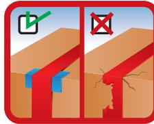
Check that securing arrangements do not damage the cargo and that the cargo doesn't damage the securing arrangements.
