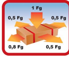
Check that the securing arrangements distribute the forces exerted by the cargo as evenly as possible and that lashings are affixed with proper angles;
