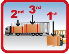
Load cargo in accordance with the planned unloading sequence;
