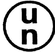
The mark is the manufacturer's certification that the battery is of a type proven to meet the test requirements of the Manual of Tests and Criteria, Part III, sub-section 38.3. This mark is not required on batteries of such a size that the mark would not be legible or to batteries not required to be of a type proven to meet the test requirements of the Manual of Tests and Criteria, Part III, sub-section 38.3."
