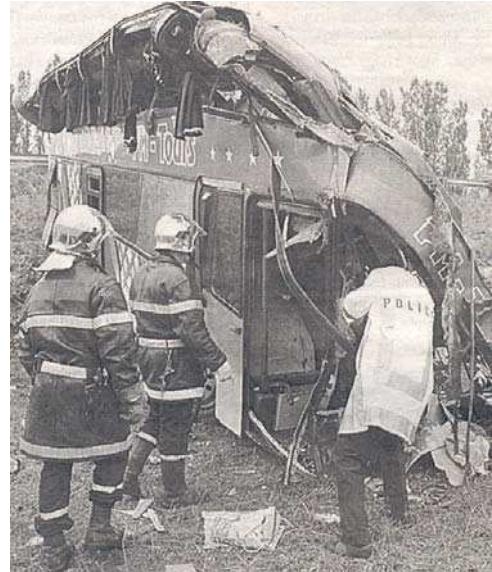
One side collapse on the UL; rigid LL, but severe damage on the driver's cab due to a frontal collision with a car
