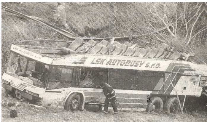
RS disappeared; UL collapsed
