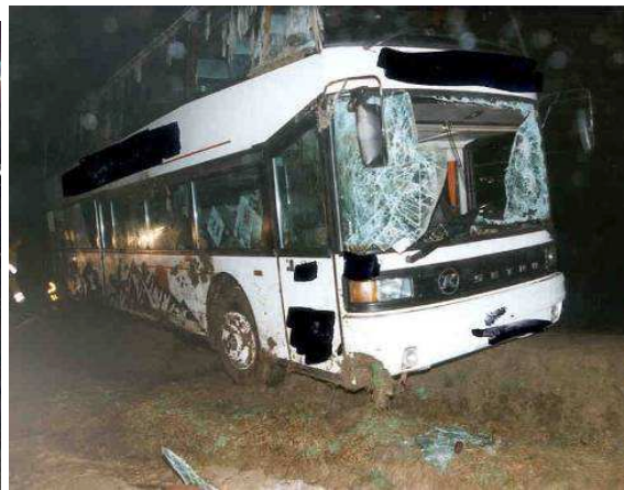
No significant deformation on the UL, rigid LL
