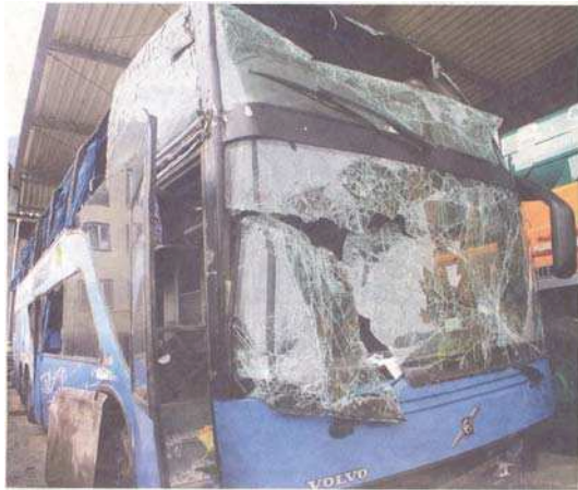
Slight deformation on the upper level (intact RS); rigid LL
