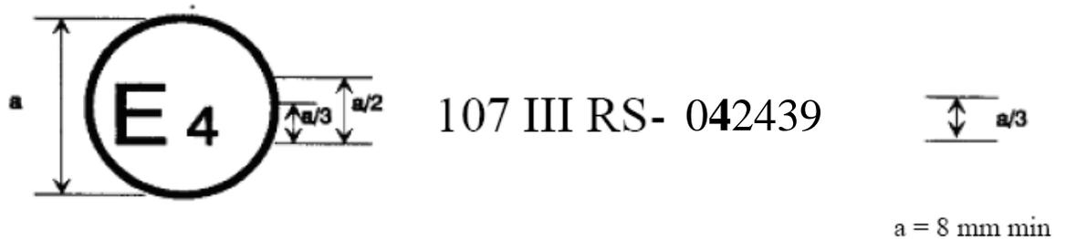
The above approval mark affixed to a vehicle bodywork shows that the bodywork type concerned has, with regard to its constructional features, been approved separately in the Netherlands (E 4) for Class III as a separate bodywork (letter S), pursuant to Regulation No. 107 under approval number 042439. The approval number indicates that the approval was granted according to the requirements of Regulation No. 107 as amended by the 04 series of amendments.”
