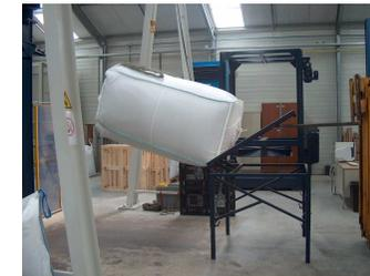
Germany is concerned that the proposed test provisions were designed for IBCs and do not readily correlate to FBCs. For example, Germany believes that it is impractical for FBCs to be tested with the proposed total test weight (6 times its gross mass--> e.g. 6 x 14 to= 78 to). Germany believes the test protocol needs to be modified to be feasible for FBCs.
