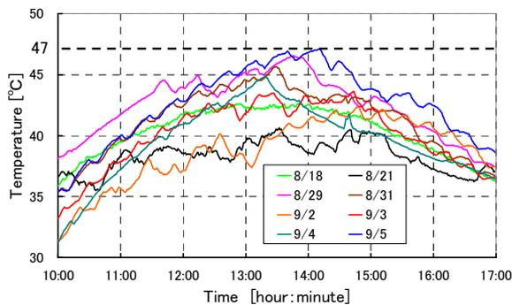
Fig.5 Temperatures on the Tank surface with sunshade
