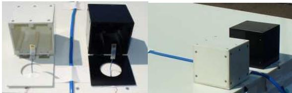
Fig.3 Boxes for comparing a temperature rise by the reflectance difference
