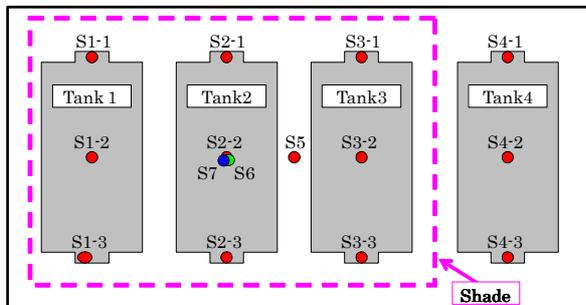
Fig.2 Temperature measurement point
