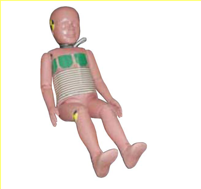
Surface pressure gauge installed on the dummy's abdomen
