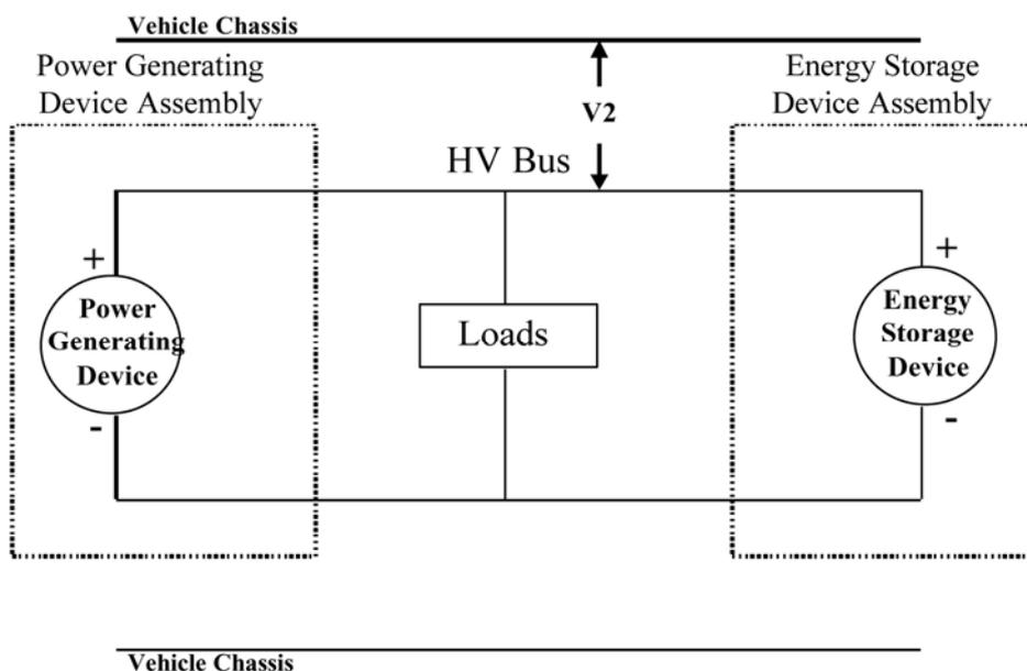
**Figure 2.2 – Measurement of the voltage between the positive side of the high voltage bus and the vehicle chassis**
