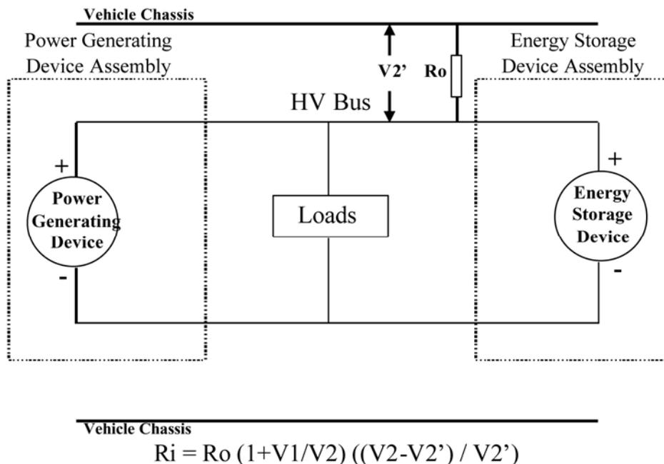
**Figure 2.4 – Voltage across resistor between negative side of the high voltage bus and vehicle chassis**
