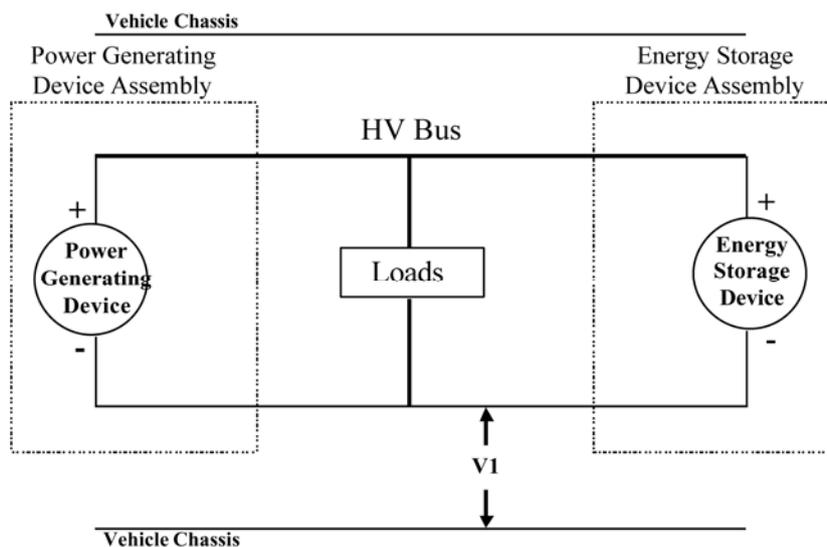
**Figure 2.1 - Measurement of the voltage between the negative side of the high voltage bus and the vehicle chassis**
