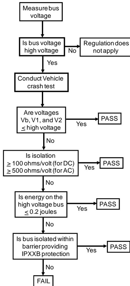
Figure 1 – Test sequence for electrical safety
