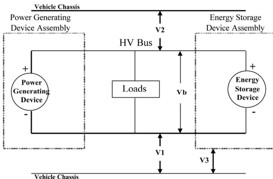
Figure 1.1 - Measurement of high voltage bus voltage
