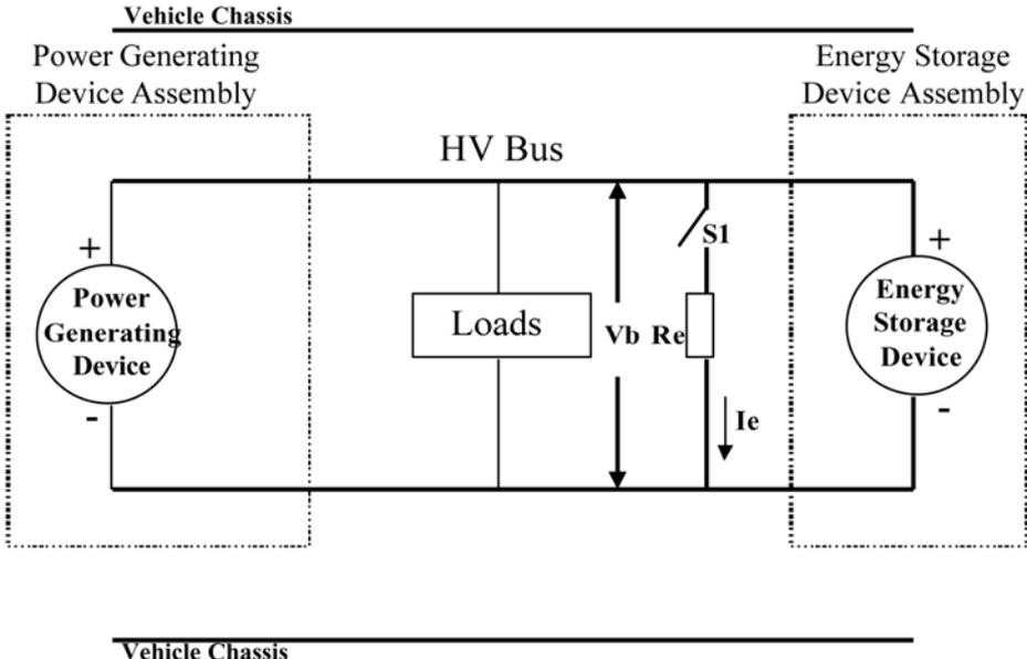
Figure 3.1 – Measurement of high voltage bus energy
