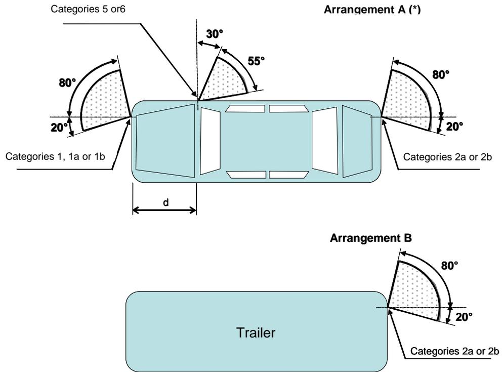
(\*) The value of 5° given for dead angle of visibility to the rear of the side-direction indicator is an upper limit.  $d \leq 1.80 \text{ m}$  (for  $M_1$  and  $N_1$  category vehicles  $d \leq 2.50 \text{ m}$ ).
