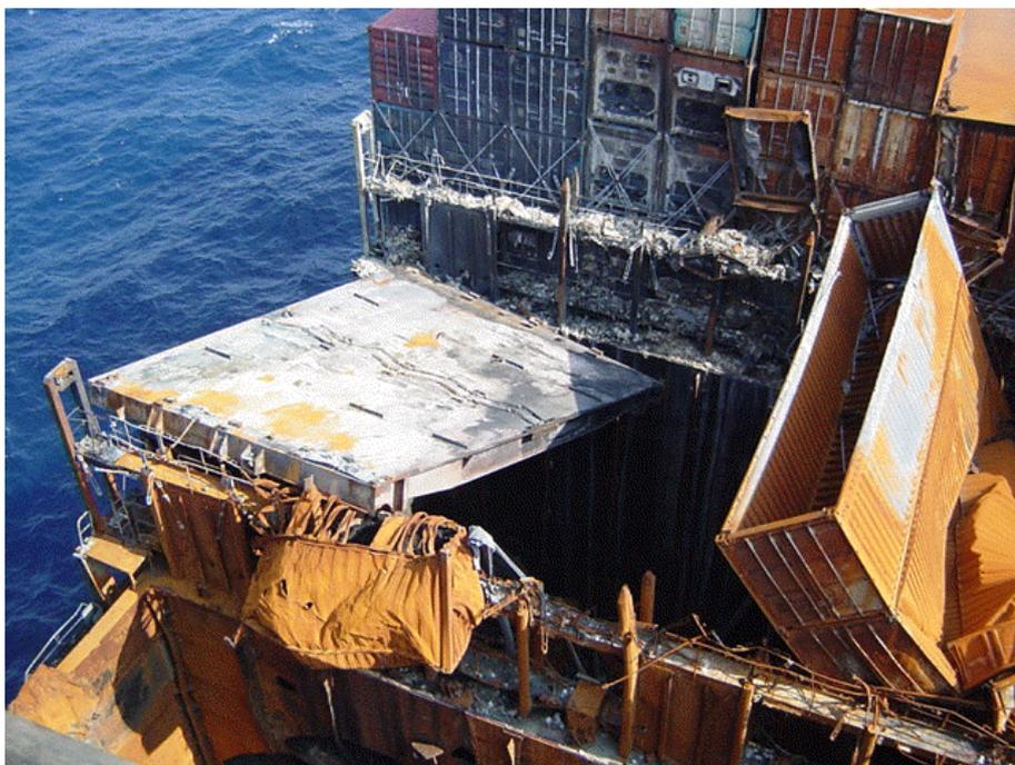
*Image 4: MV Hanjin Pennsylvania – damage to hatch covers*
