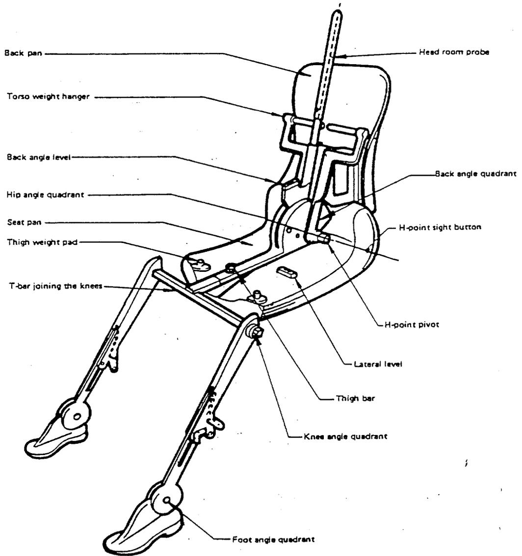
Figure 1 - 3-D H machine elements designation
