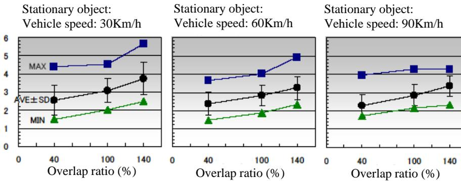
The minimum value of these values (the minimum value of the steering start timing) is regarded as the threshold value.
