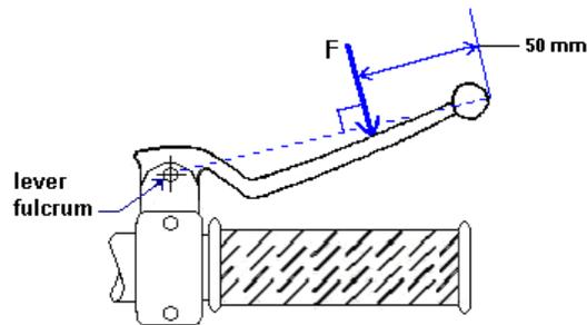
The input force is applied to a point located 50 mm from the outermost point of the control lever, measured along the axis between the central axis of the fulcrum of the lever and its outermost point.
