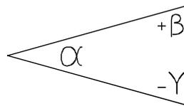
where  $\alpha$  is the angle measured from the horizontal position of the front face (fitted the right way up) of the equipment for which the instrument is calibrated, while  $\beta$  and  $\gamma$  represent respectively the maximum permissible upward and downward deviations from the angle of calibration  $\alpha$ .
