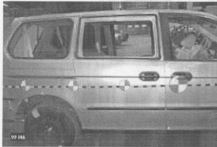
Outside view of the sliding door, pre-test
