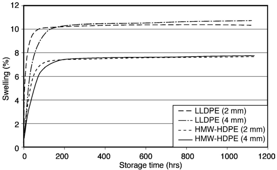
Fig 5 Swelling of HMW-HDPE and LLDPE material as a function of storage time for 2 thicknesses in xylene mixture at 40°C
