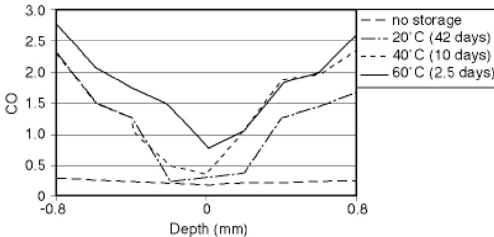
Fig 3 Amount of carbonyl (C=O) as a function of cross-section depth
