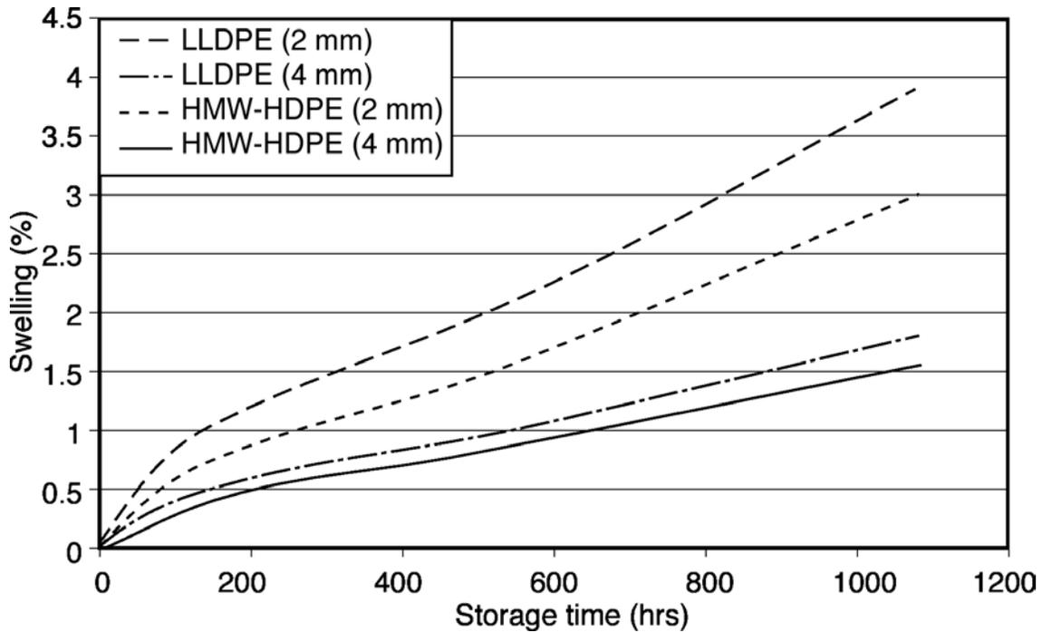
Fig 6 Swelling of HMW-HDPE and LLDPE material as a function of storage time for 2 thicknesses in aliphatic mixture at 23°C
