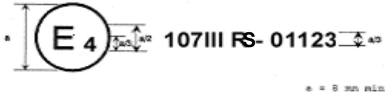
The above approval mark affixed to a vehicle bodywork shows that the bodywork type concerned has, with regard to its constructional features, been approved separately in the Netherlands (E 4) for Class III as a separate bodywork (letter S), pursuant to Regulation No. 107 under approval number 01123. The approval number indicates that the approval was granted according to the requirements of Regulation No. 107 as amended by the 01 series of amendments.
