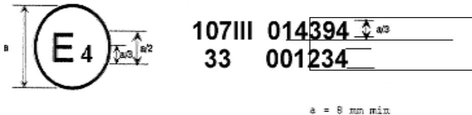
The above approval mark affixed to a vehicle shows that the vehicle type concerned has been approved in the Netherlands (E 4) pursuant to Regulations Nos. 107 and 33.\*/ The first two digits of the approval numbers indicate that, at the dates when the respective approvals were given, Regulation No. 107 included the 01 series of amendments and Regulation No. 33 was in its original form.
