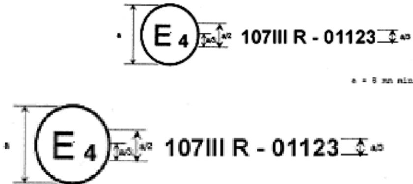
The above approval mark affixed to a vehicle shows that the vehicle type concerned has, with regard to its constructional features, been approved in the Netherlands (E 4) for Class III, pursuant to Regulation No. 107 under approval number 01123. The approval number indicates that the approval was granted according to the requirements of Regulation No. 107 as amended by the 01 series of amendments.
