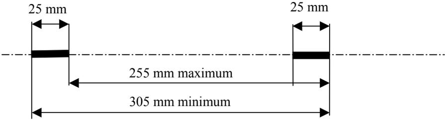
Figure 4: Distance between both low anchorage zones
