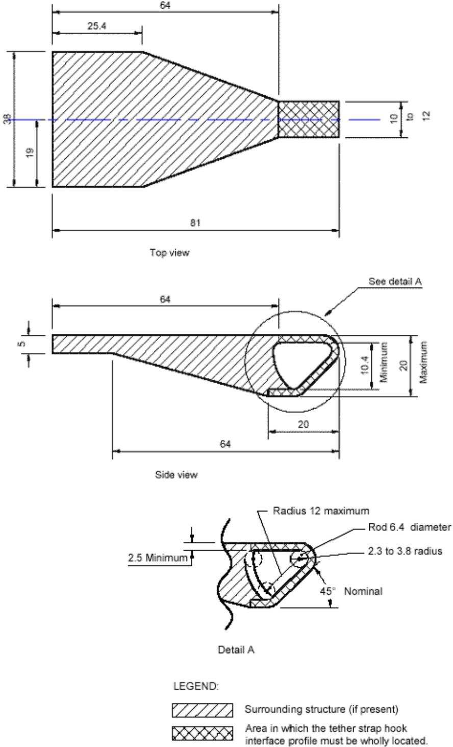
Figure 3: ISOFIX Top tether connector (hook type) dimensions
