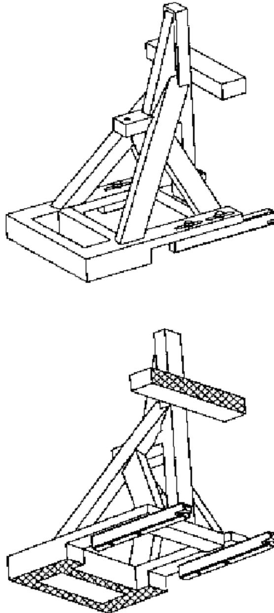
Figure 1: Static force application device (SFAD), isometric views
