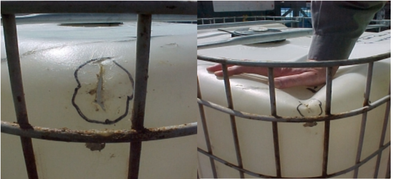
Damage to corner of IBC (inside undamaged outer package corner) stemming from upper pallet base coming into contact with rigid plastic inner package.
