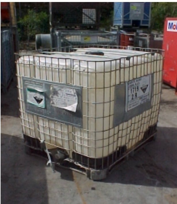
Light weight IBC with minimum outer packaging, particularly on the upper surface, and specially designed pallet base
