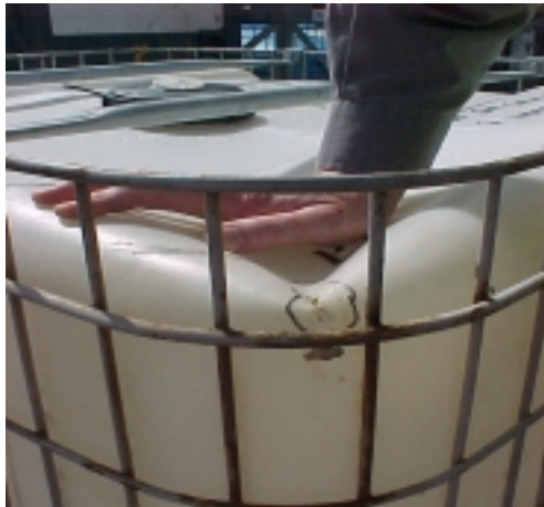
Compressive damage has occurred despite cross rails and frames being undamaged. This IBC has been certified as a reusable IBC without restriction.
