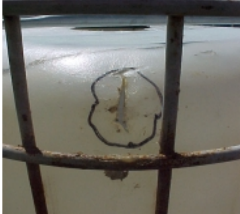
Damage to corner of IBC (inside undamaged outer package corner) stemming from upper pallet base coming into contact with rigid plastic inner package.
