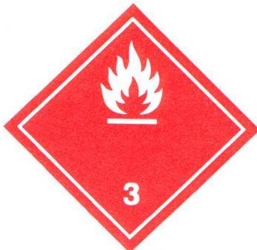
**Pictogram for flammable liquid in the UN Model Regulations (Symbol: Flame: Black or White; Background: red; Figure 3 in bottom corner; minimum dimensions 100 mm x 100 mm.)**
