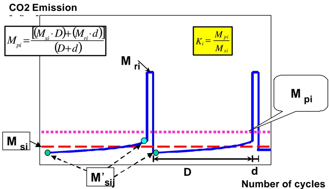
**Figure 8/1:** Parameters measured during carbon dioxide emission and fuel consumption test during and between cycles where regeneration occurs (schematic example, the emissions during 'D' may increase or decrease)
