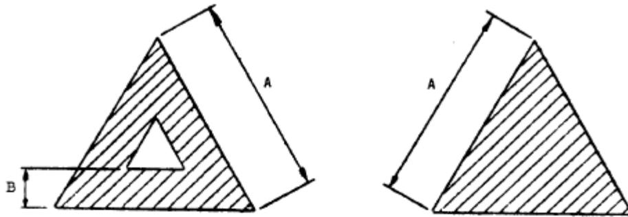
$$\begin{aligned} 150 \text{ mm} &\leq A \leq 200 \text{ mm} \\ B &\geq \frac{A}{5} \\ C &\leq 15 \text{ mm} \end{aligned}$$
