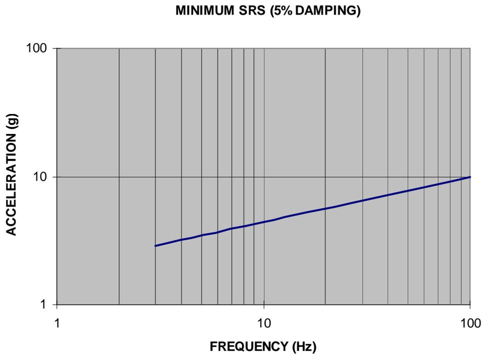
Equation for generating the above Minimum SRS Curve:  $ACCEL = 1.95 \text{ FREQ}^{0.355}$
