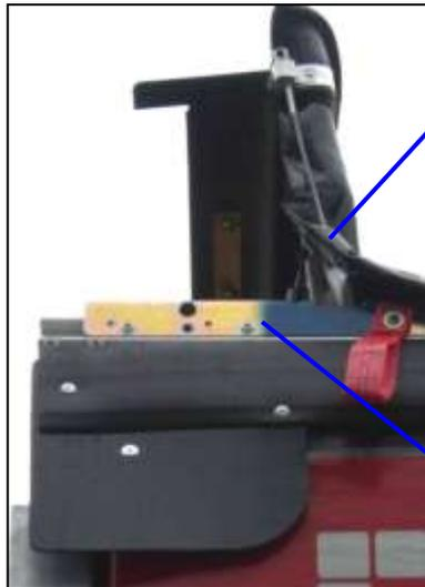
Tensioning device on the lever mechanism. By folding down the tensioning device, the steel rope will tension.
