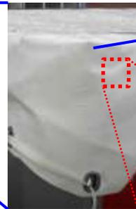
The fixing point of the fastening steel rope is completely covered and secured by the roof curtain.
