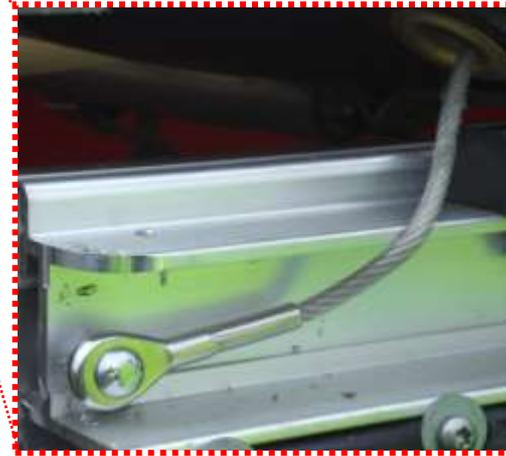
Detail photo from the fixing point of the fastening steel rope at the front.
