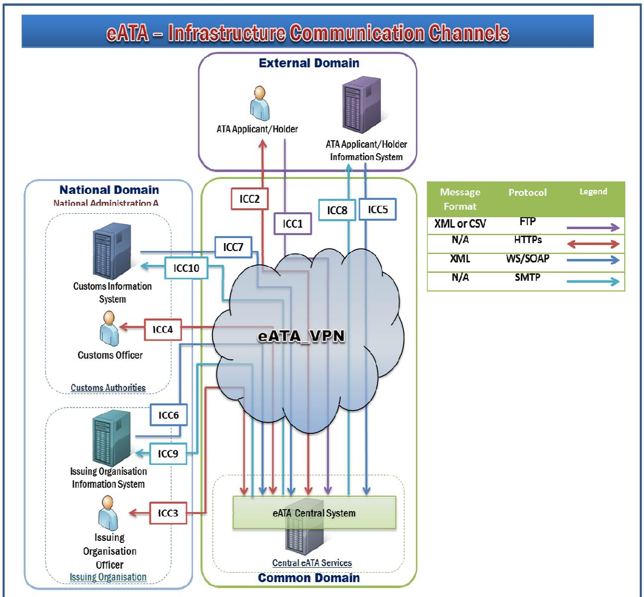
Figure 2-3: Overview of Infrastructure Communication Channels
