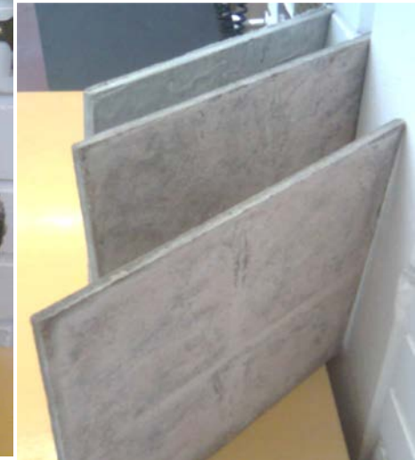
GRP waste fibre filled cement composites Produced panels: (30x30 cm) 8 & 12 mm thick
