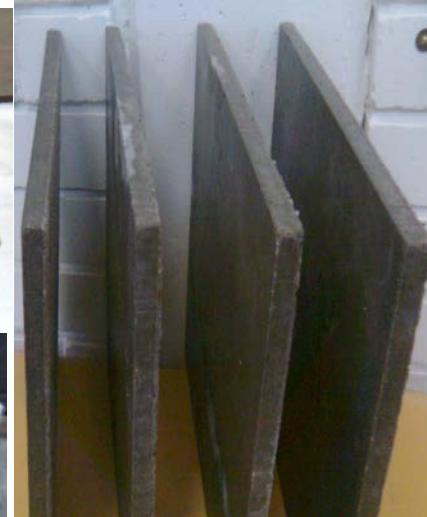
GRP waste fibre filled cement composites Produced panels: (30x30 cm) 8 & 12 mm thick
