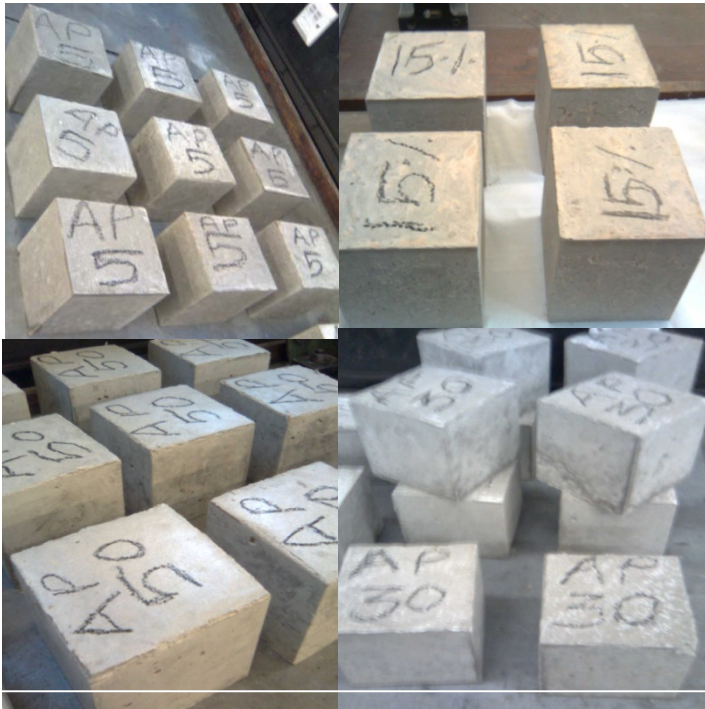
190 GRP waste powder filled concrete composite specimens
