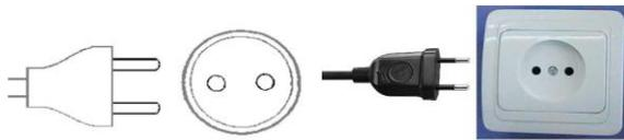
This two-wire plug is ungrounded and has two round prongs. It is popularly known as the europlug which is described in CEE 7/16. This is probably the single most widely used international plug. It will mate with any socket that accepts 4.0-4.8 mm round contacts on 19 mm centres
