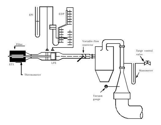
4.2.4.3. A CVS system that has multiple speeds shall be calibrated on each speed used. The calibration curves generated for the ranges shall be approximately parallel and the intercept values  $(D_0)$  shall increase as the pump flow range decreases.
