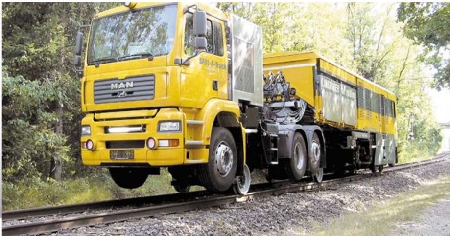
RAIL/ROAD TRUCKS FOR RAIL MILLING AND GRINDING
