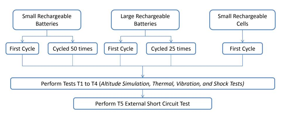
All tests T1 to T5 are currently performed only with un-cycled cells
