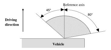
Under the H plane for front position lamps intended to be installed with this plane at a mounting height less than 750 mm above ground.
