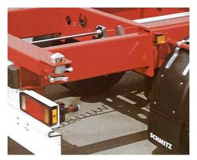
Figure 2.1 Twistlock on a road vehicle
