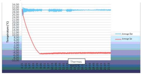
Example of a cool-down test recording
