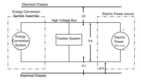
Figure 1: Measurement of Vb, V1, V2, V3
