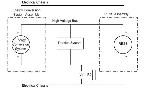
Figure 3: Measurement of V'1
