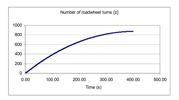
This measurement was done until  $t_{\Sigma}$ , total deceleration time, to check the result obtained.
