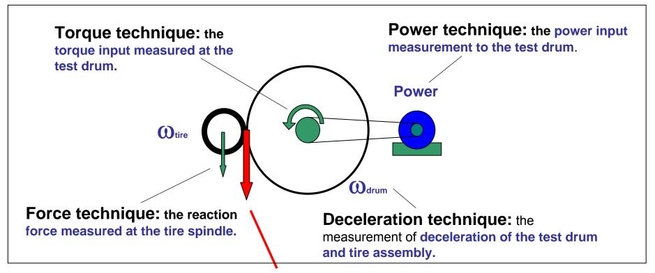
For each technique, the test results are converted to the force acting at the tire/drum interface, which is the tyre rolling resistance.
